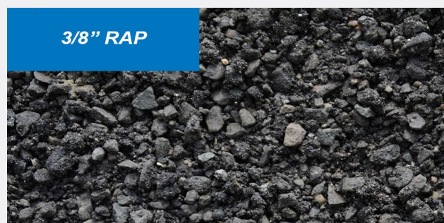
Caption: Example material in a RAP stockpile
